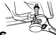
If washer is not level, screw the front legs up or down to adjust. Repeat Step 15.
